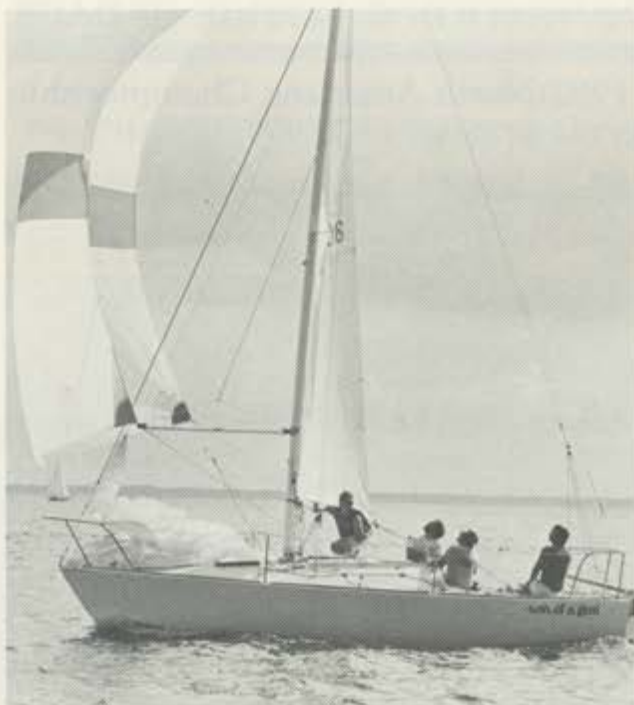
Proper spinnaker trim means level clews.
