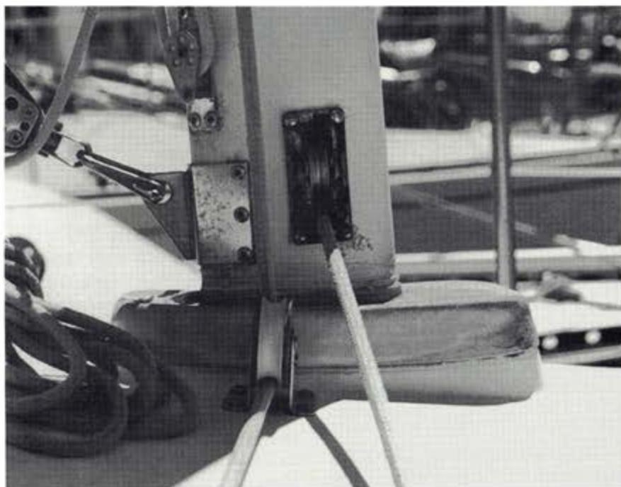
Above, if your mainsail halyard exits at deck level, you should be extra diligent in looking for cracks. The six vang fitting rivets and the big square hole for the exit sheave weaken the mast at this highly-stressed location. Below, a burr here in the sheave box will eat up halyards faster than you can replace them.
