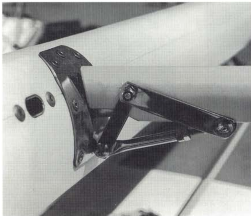
Above, this photo shows a Proctor mast. The spreaders have been epoxied into the bracket. Below, this Kenyon spar has been retro-fitted with a thru bar and also has had spreader adjusters installed. The rivets in the spreader plate and the Gibb fitting below it should be checked annually and repairs made if they are loose.
