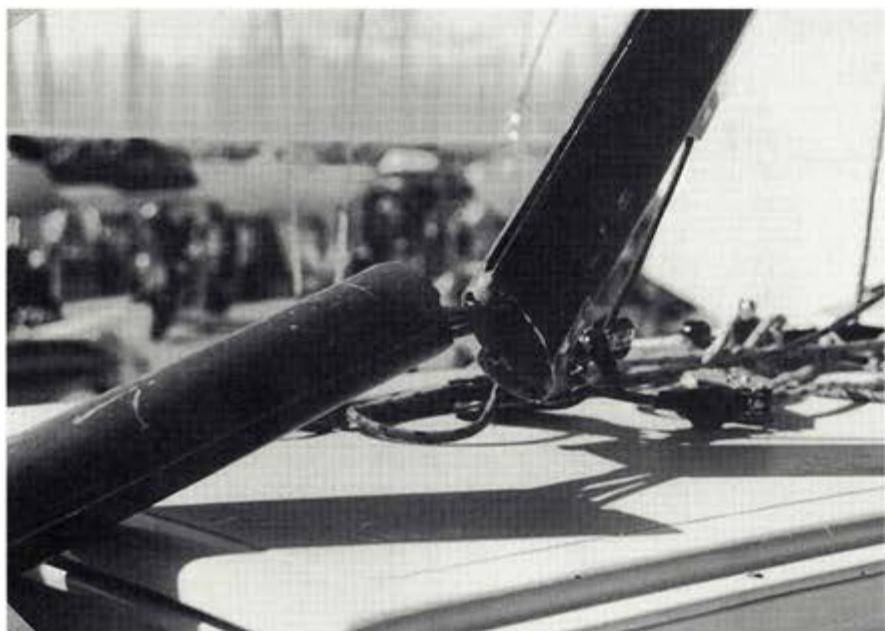
Above, the broken boom that nearly cost Ken Read the title. Read's crew rejected a spinnaker pole the day before race one when they found corrosion and pitting under some tape. They were looking for problems but this one escaped their attention.
