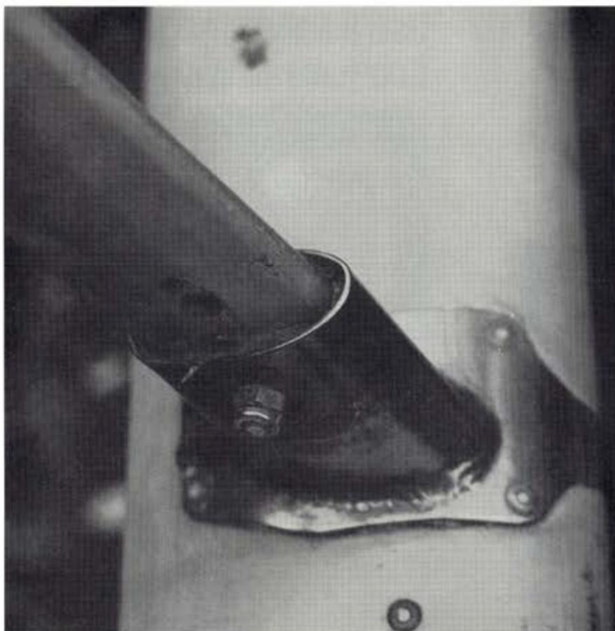
Above, this photo shows a Proctor mast. The spreaders have been epoxied into the bracket. Below, this Kenyon spar has been retro-fitted with a thru bar and also has had spreader adjusters installed. The rivets in the spreader plate and the Gibb fitting below it should be checked annually and repairs made if they are loose.
