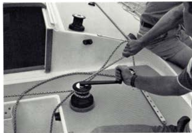
4. Finally, the helmsman places the handle into the winch and makes final genoa adjustments.
