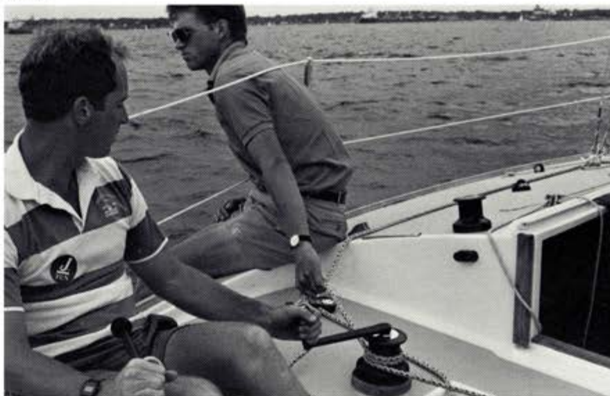
For upwind trimming, cross sheeting enables the helmsman to fine tune genoa trim through puffs and waves. Here the genoa sheet is rarely cleated upwind.
