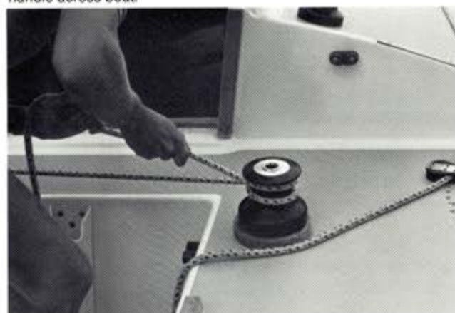
3. Once genoa is almost fully in, jibman quickly places additional wraps on winch on his way to the windward rail
