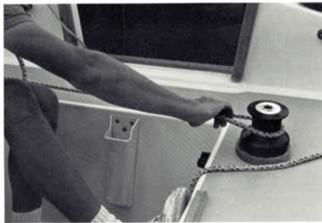
2. Jibman moves straight across cockpit, places a half wrap around the new windward winch, and takes full length arm pulls.
