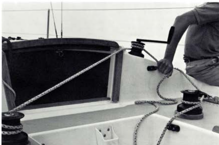
If the jib trimmer is more comfortable with the leeward sheeting method, then fine adjustments can be made by leading the sheet around the windward halyard winch. Notice that weather sheet is pre-wrapped around unused winch in preparation for a tack.
